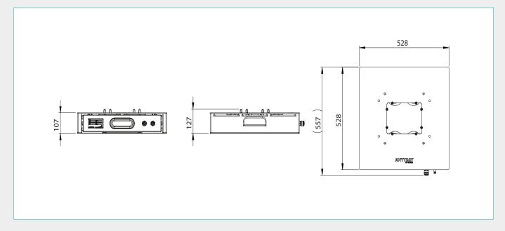
Specifications and photos are intended as a guide and can be changed by QUPAQ without notice. We make reservations for misprints and typing errors. The illustration and specifications are of the ANYTRAY LeanOne Tool - Buffer. Item no. 91300028.
