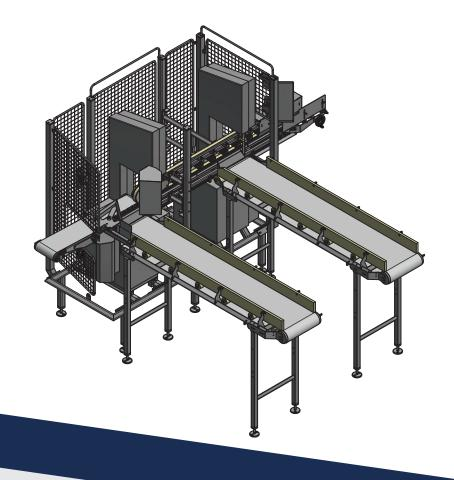
Automatic cutting of rib plates which can be divided into 2: loin rib. The machine is fully flexible so product widths can be adjusted, and one saw can be easily deactivated If only 1 cut is needed.
