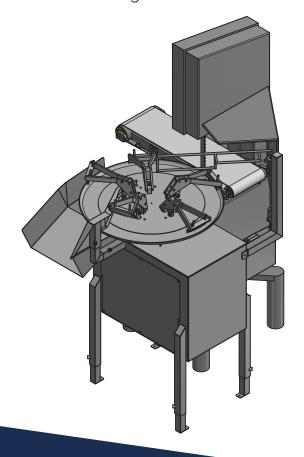
Pork Neck bones are manually placed on the product feeding round table and are held accordingly during the automatic sawing process. The two sawed products are guided away and ready for next processing or packaging.
