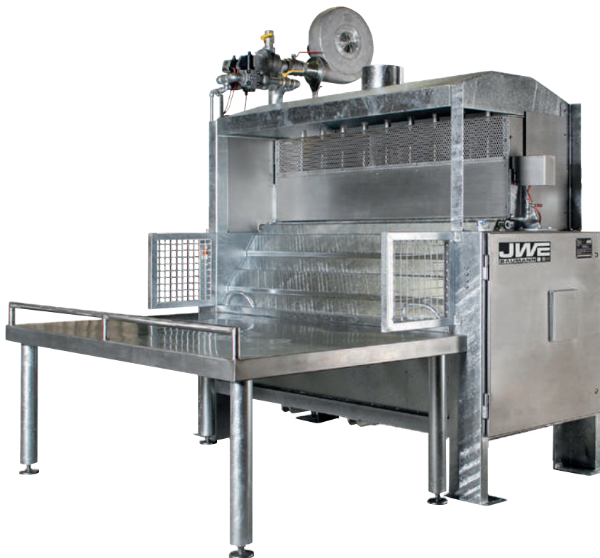
Fig. with natural gas singeing and ejection table
