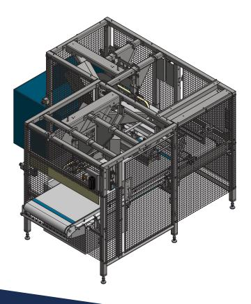
To ensure a higher profit for bacon, pork belly's are automatically cut on two sides into a square figure. This results in a more uniform width of the sliced bacon products. The size of the square can easily be adjusted to needed width of the following sliced bacon.
